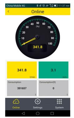
Please download the service app from the Google Play in case you need to have any settings changed on the S 415. The app is running on any Android system with BlueTooth support. To change settings the app needs to scan the QR code on the calibration certificate at first. This ensures that only valid users can access the sensor settings. Follow the instruction in the service app.
