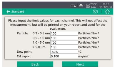
The user has to define the limits values for each measurement channel when selected CLASS 0. By this the user is able to select different alarm settings as needed by the quality management.
