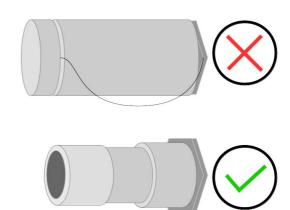
Remove the protection caps from all parts of both sides of the instrument. If not removed the device may get damaged and its the risk of bursting parts under high pressure, this can lead to a damage or to personal injuries. All exhaust outlets will pass air during the measurement, if not, please contact the manufacturer.
