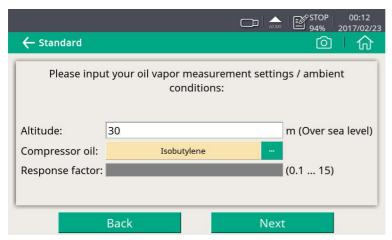
The ambient conditions like the sea level are needed to be defined. Also the oil type can be selected (Isobutylene is recommended as this will meet the most oil characteristics).
