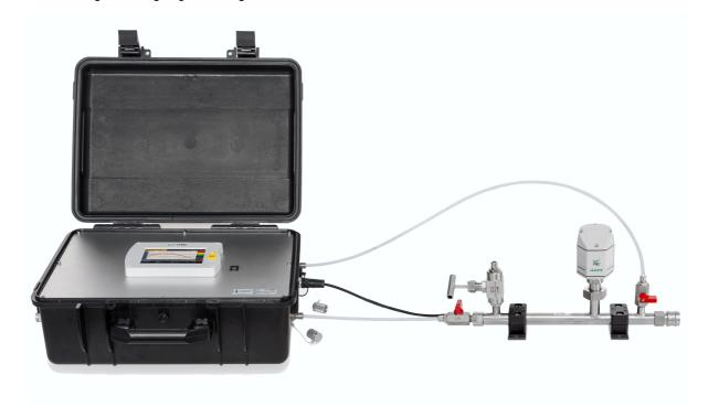
The picture above shows the setup together with the isokinetic sampling device connected to the S 600. Please connect the isokinetic sampling device using the teflon hose which came with the device. On the next page you will find a detailed description of the sampling device. Also you will find which outlets of the sampling device need to be connected to which input at the S 600.
