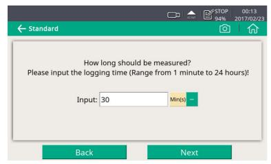
It has to be defined how long the measurement should take. The longer it takes, the more the values are stabilized and represent the system conditions exactly.
