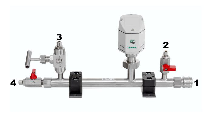
Before connecting you compressed air, make sure ball valve **2 and 4 are closed** properly.
