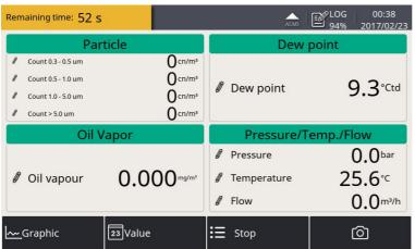
Measurement has started. Logging is indicated by the pens moving on the screen. Also the status bar icon switches from STOP to LOG. The remaining time is displayed in the upper left corner. Please wait. The system will stop the measurement automatically.
