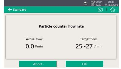
Set up the flow rate shown on the screen.
