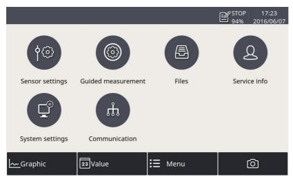
The user can get to the main menu by pressing the menu bar in the bottom bar. From here the user can get to different sub-menus like the guided measurement or the system settings.
