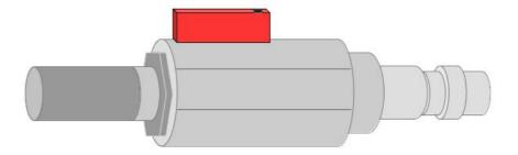
To check your point of measurement connect the purge filter test it onto your measuring point first. Open the purge valve on the test kit and purge some air for a short period. Afterwards check the filter in the test kit, if it shows high contamination of water, oil or dust. Should the filter be contaminated to high do not continue to measure with the S 600 as this may lead to serious damage. In case you are not sure, please contact the manufacturer.
