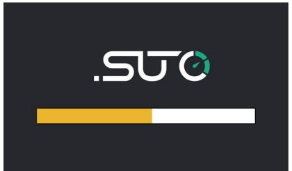
When the S 600 gets powered you will see the start up screen. The progress bar shows, that the sensors are configured and the device is running some initialization routines.
