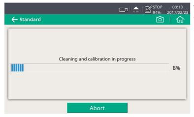
The system is performing the self calibration cycles and is cleaning the internal sensor elements.
