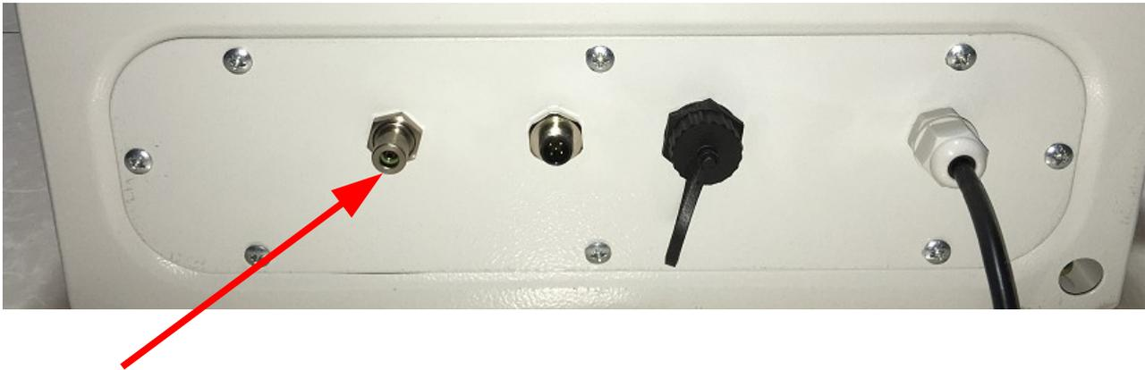
The S 601 has a compressed air input on the lower side of the cabinet next to the electrical connections.
