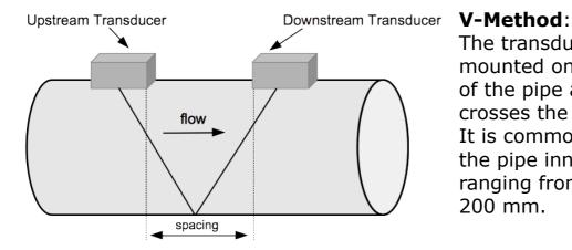
The transducers are mounted on the same side of the pipe and the sound crosses the pipe twice. It is commonly used when the pipe inner diameter ranging from 15 mm to 200 mm.
