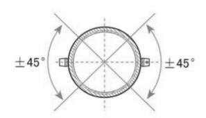
If the Z-Method is used, make sure that the transducers are mounted on a pipe within a valid angle range, as shown in the left picture.
