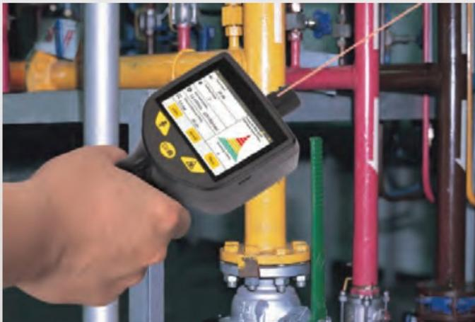
3. Point at a suspected leak with the laser. The leakage grade and leak amount are shown on the touch screen.
