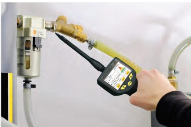
5. When you are close to the leak point, mount the focus tube and focus tip onto the sensor, and scan with the focus tip until the exact location is found.
