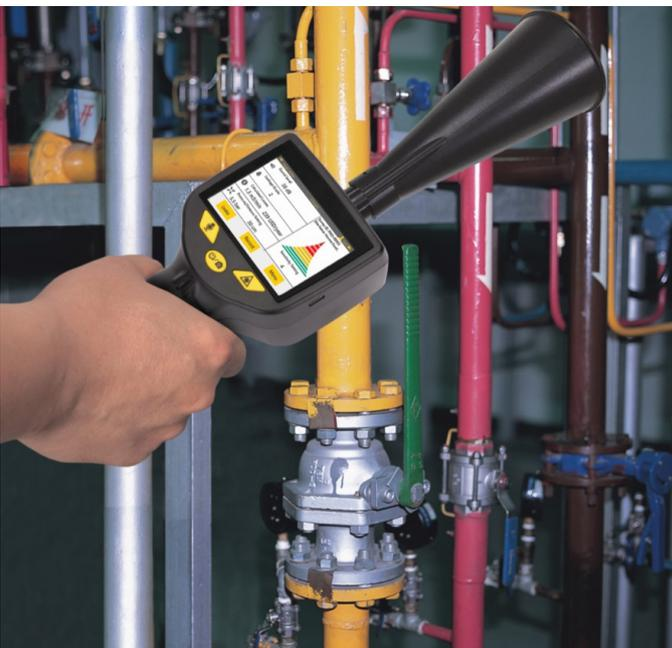
4. Mount the trumpet on the sensor and locate the rough leak range.
