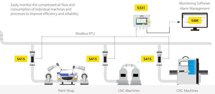
S415 Compact Thermal Mass Flow Meter (Eco-Inline)
